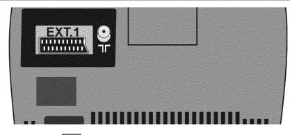
**EXT.1** Scart socket: To connect a satellite receiver, decoder, video recorder, etc.
